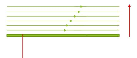
Velocities of layers increases as distance from the fixed surface increases
